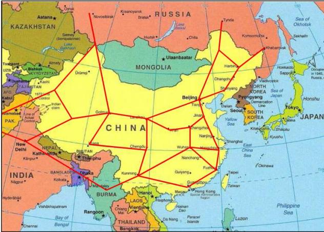
Figure 6: Proposed HVDC Grid for Continental Asia Connections to Europe via HVDC lines along the Trans-Siberian Railway (Figure 7) and on to Africa (routes not shown in meaningful detail; meant to illustrate the concept).
