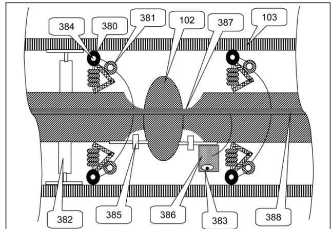
Figure 9: Splice Module and Carriage Details
