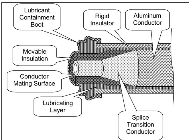
**Figure 4: Rigid Insulation for Elpipe Segment**
