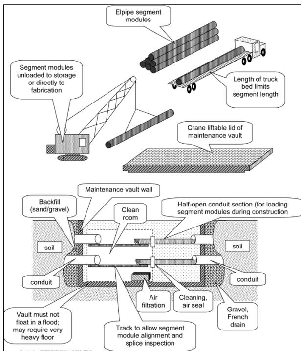
Figure 8: Installation and Maintenance Vaults
