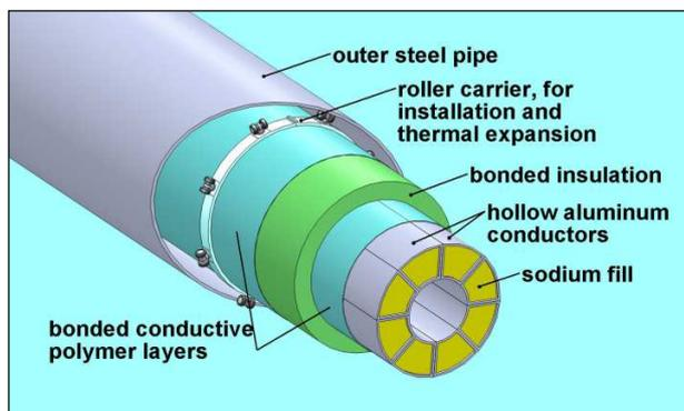
Figure 1. Cutaway view of elpipe segment module
