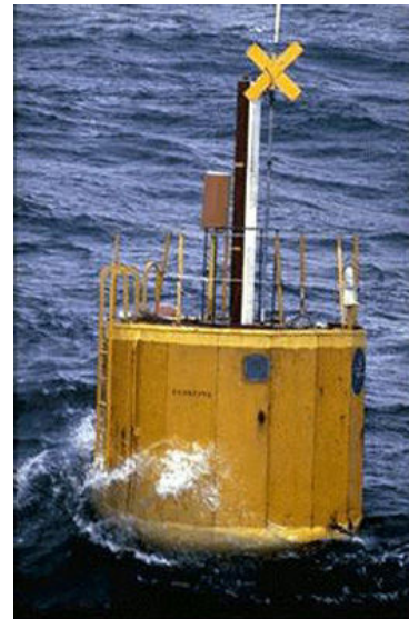
Picture 8: The AquaBuOY in operating
