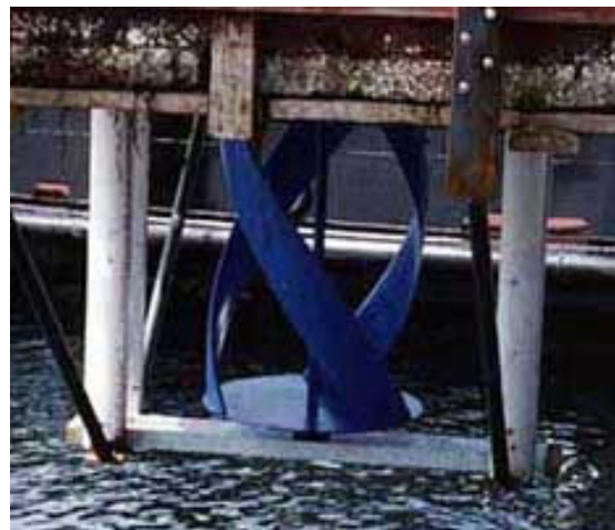
Picture 3: Vertical axis turbine in commissioning
