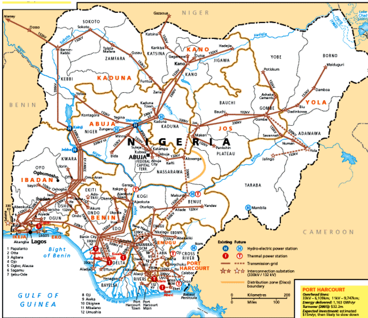
Figure 3 Nigeria's power grid Source: Google
